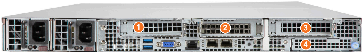
Figure 3-11. PCI Expansion Card Chassis Slots
