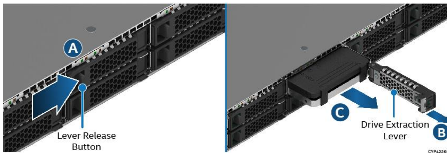
Figure 38. 2.5" 7 mm Drive Removal
