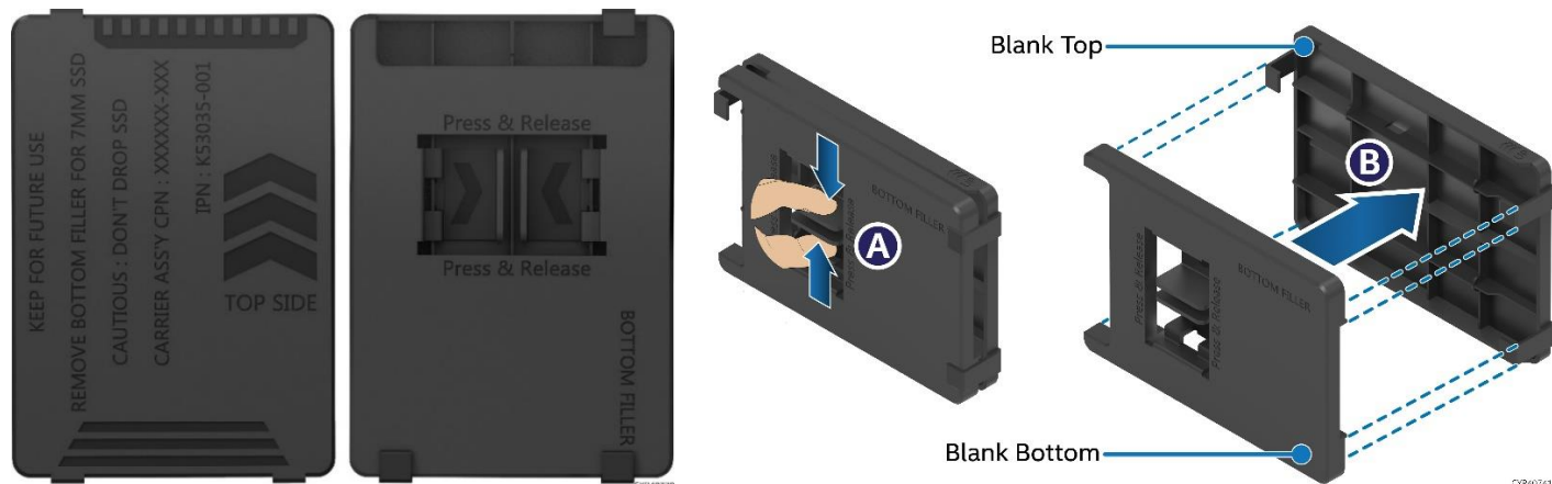
Figure 99. Separating Top and Bottom Parts of Drive Blank
