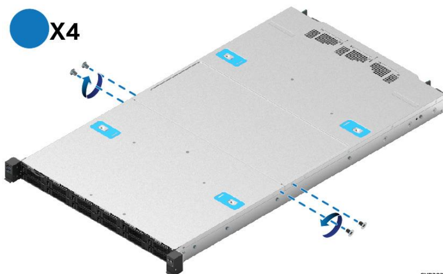
Figure 19. System Top Cover Panel Shipping Screws
