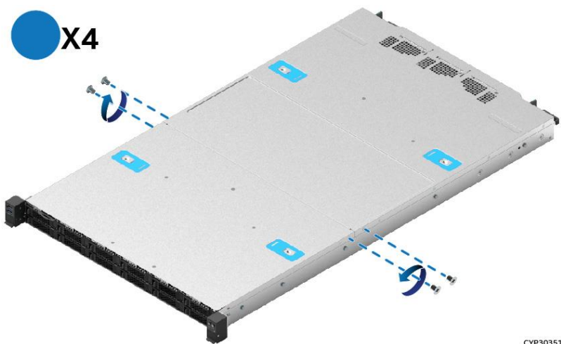
Figure 74. System Top Cover Panel Shipping Screws
