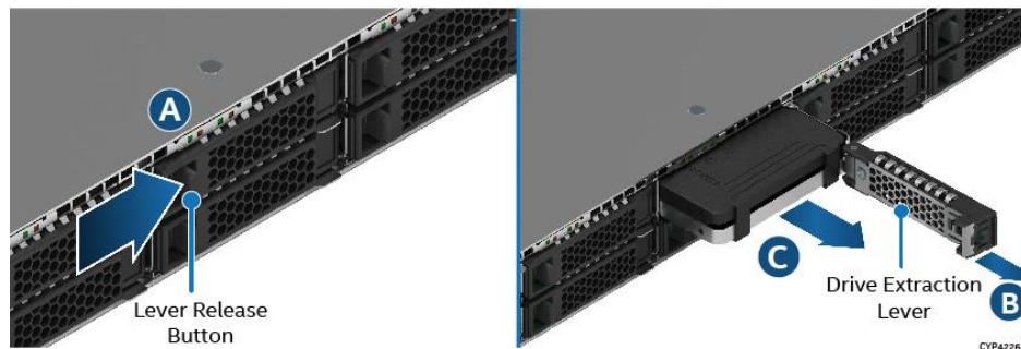
Figure 97. 2.5" 7 mm Drive Removal
